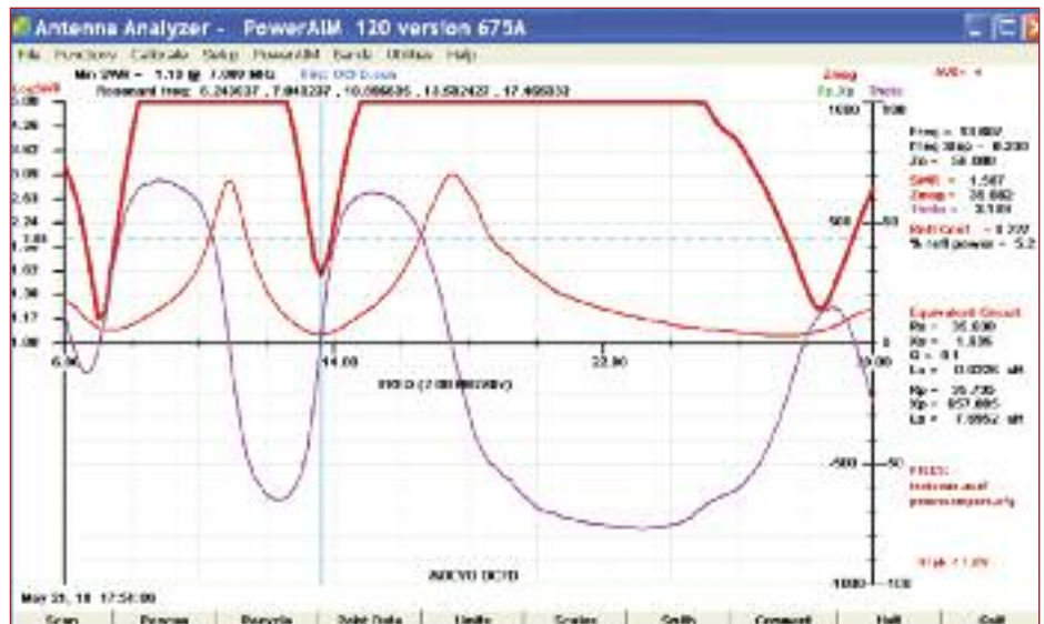
FIGURE 4: Impedance and SWR measurements of the MOCVO HW-40HP antenna, measured using the AIM 4170.
